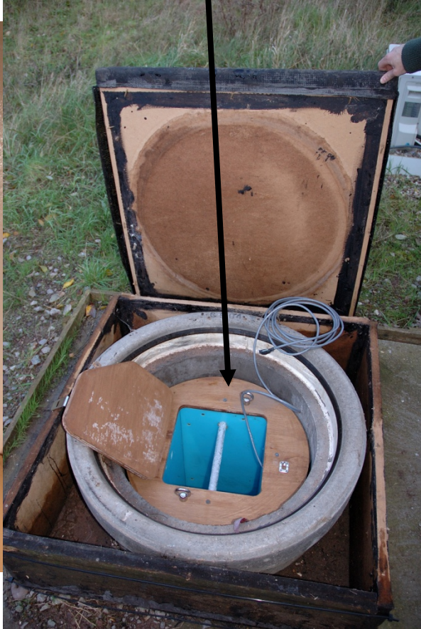
Pit for long terms offset and noise measurement
