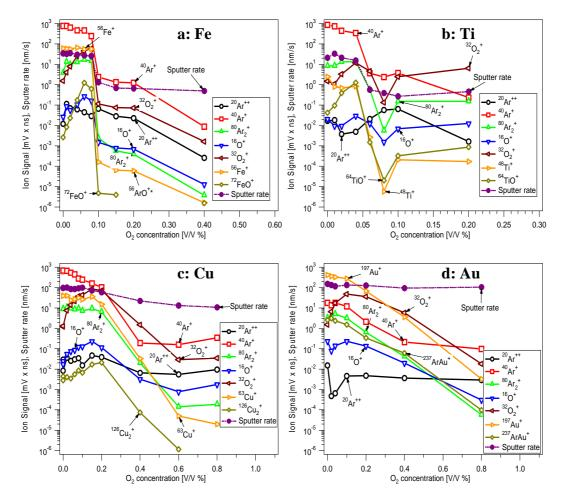
Fig 5. Ion signals and sputter rates vs. oxygen concentration for samples of *a*: Fe, *b*: Ti, *c*: Cu, *d*: Au. The voltage was 700 V and the current 20 mA in all cases.
