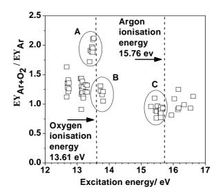
Fig. 4: Plot of EY ratios of all observed Fe II lines plotted against total excitation energy for 0.20 %  $O_2$  for 700 V and 40 mA.
