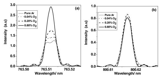
Fig. 3 Example of line profiles of (a) Ar I 763.511 nm, showing self-absorption and (b) Ar I 800.616 nm for various O<sub>2</sub> concentrations. Discharge conditions were 700 V, 20 mA for a 4 mm anode tube diameter.
