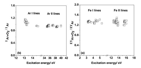
Fig. 2 (a) Intensity ratios (R<sub>I</sub>) of Ar I and Ar II vs. total excitation energy (TEE) and (b) Emission yield ratios (R<sub>E</sub>) of Fe I and Fe II lines; 700 V and 20 mA and 0.04 % v/v oxygen concentration.
