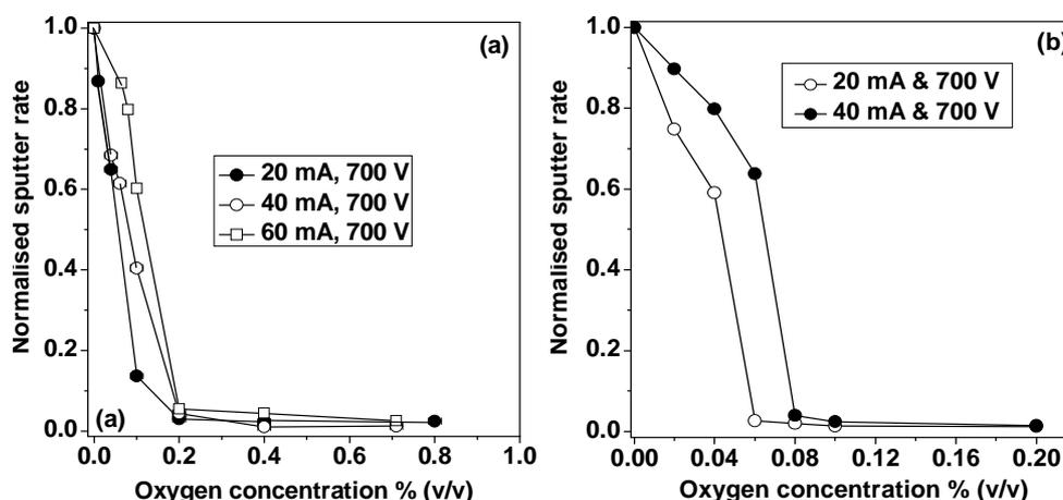
Fig. 1 Normalised sputter rate for (a) iron and (b) titanium as a function of oxygen addition at 700 V and different currents in 4 mm anode tube.
