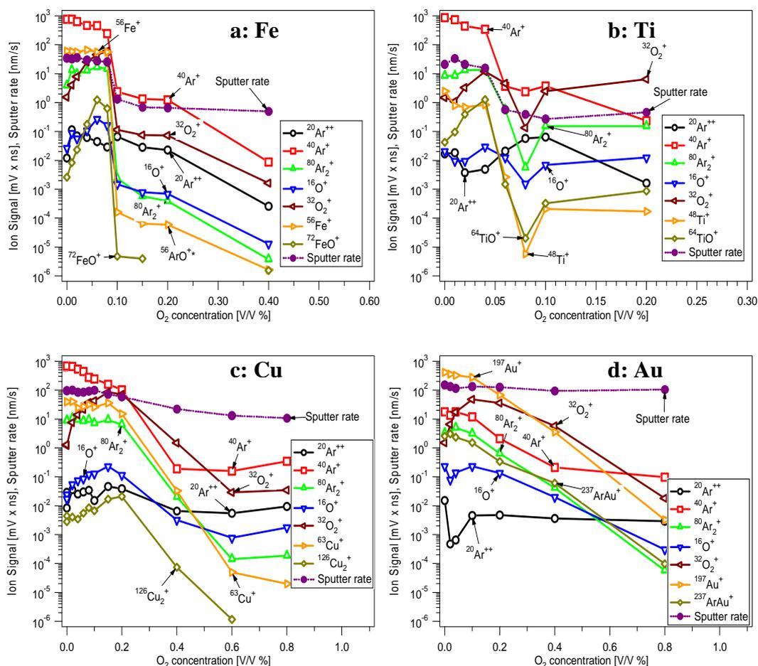
**Fig 5.** Ion signals and sputter rates vs. oxygen concentration for samples of *a: Fe, b: Ti, c: Cu, d: Au*. The voltage was 700 V and the current 20 mA in all cases.
