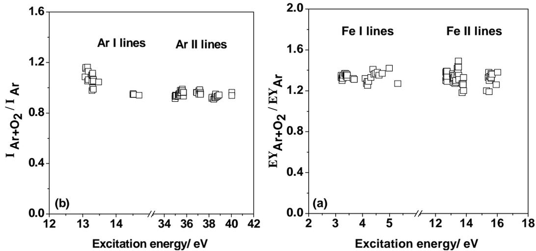
Fig. 2 (a) Intensity ratios ( $R_I$ ) of Ar I and Ar II vs. total excitation energy (TEE) and (b) Emission yield ratios ( $R_E$ ) of Fe I and Fe II lines; 700 V and 20 mA and 0.04 % v/v oxygen concentration.
