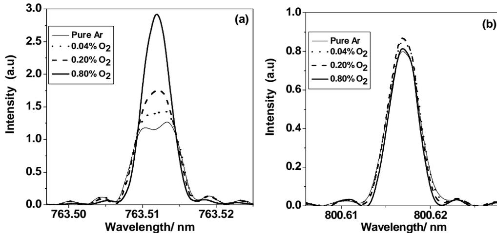
Fig. 3 Example of line profiles of (a) Ar I 763.511 nm, showing self-absorption and (b) Ar I 800.616 nm for various  $O_2$  concentrations. Discharge conditions were 700 V, 20 mA for a 4 mm anode tube diameter.
