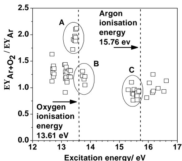
**Fig. 4:** Plot of EY ratios of all observed Fe II lines plotted against total excitation energy for 0.20 % O<sub>2</sub> for 700 V and 40 mA.
