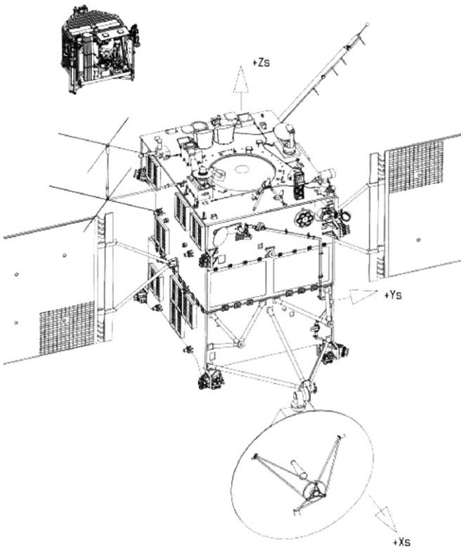
**Fig. 2.** Schematic diagram of the Rosetta spacecraft (adapted from [Accomazzo et al., 2010](#)). Most instruments are on the +Z-panel and were pointing towards Lutetia during the flyby. The Lander is attached to the -X-panel with Ptolemy Vent pipe pointing towards Lutetia and COSAC vent pipe pointing away from Lutetia.
