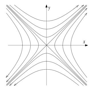
(c) The magnetic pressure is defined as  $p_B = \frac{B^2}{2\mu_0} = \frac{(B_0 y)^2 + (B_0 x)^2}{2\mu_0} = \frac{B_0^2}{2\mu_0} \left(x^2 + y^2\right)$
